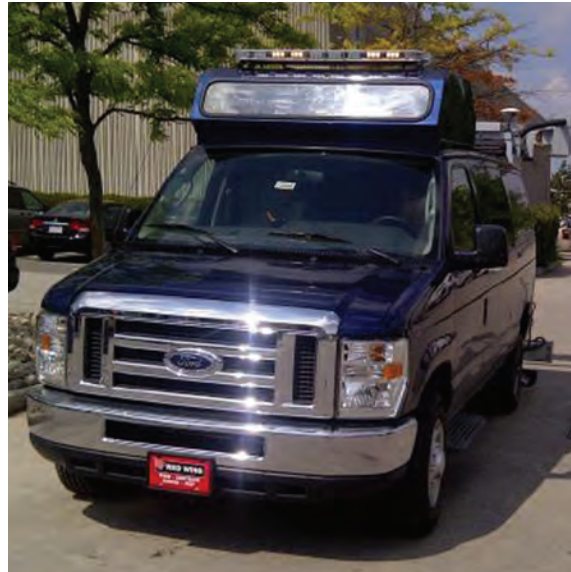
The SDDOT's state-of-the-art roadway data acquisition van travels every mile of state highway every year to collect data and images.
