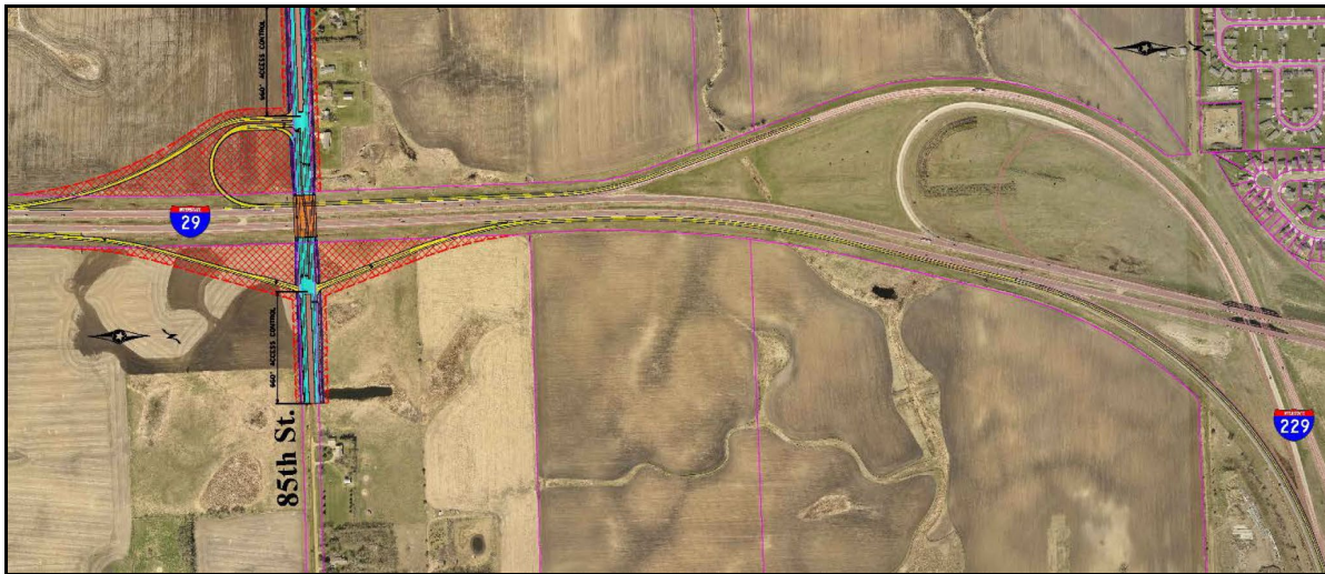
Figure 2-5: IJR Folded Diamond Interchange (Previously Dismissed)
