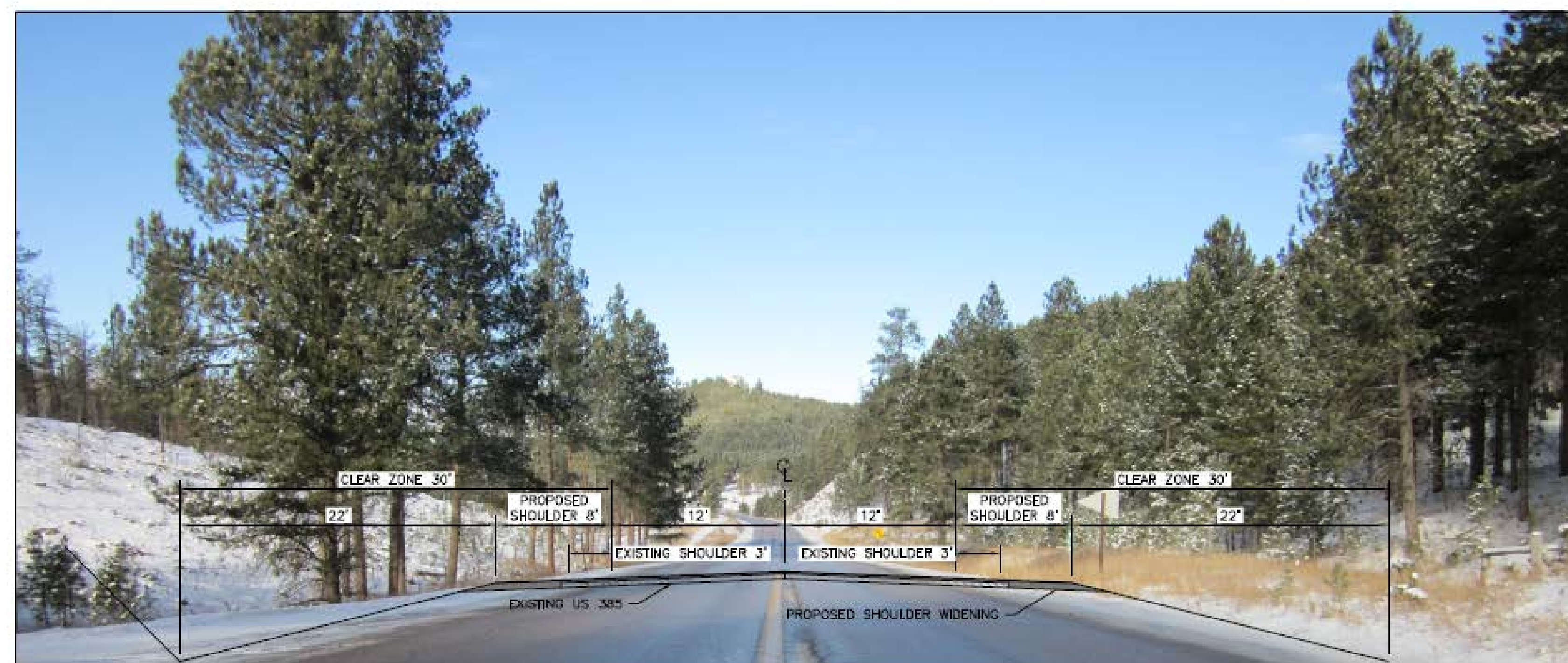
TYPICAL SECTION (SHOULDER WIDENING) MRM 96,657 TO MRM 102,37
