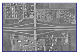
queuing problem will continue. It may be desirable to construct a separate right turn lane on the westbound off-ramp to increase the capacity and storage length available on the ramp.
