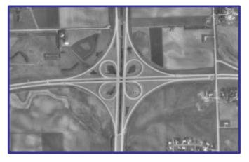
provided between the loop ramps does not meet current design criteria. The other geometric deficiencies are relatively minor, and can be corrected at the time of reconstruction. In an effort to address the geometric issues, a full cloverleaf interchange that meets current design criteria was developed for this system interchange. The results of the Phase II investigation are summarized below along with selected information from the Exit 395 Phase I analysis.
