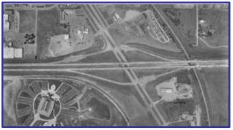
additional traffic signals will likely be required along the corridor. Consideration should be given to reconstructing the interchange with a single point configuration, which would increase the signal spacing from approximately 450′ between the northern ramps and the next major intersection, to approximately 800′. If reconstructed, the relatively minor geometric deficiencies could be addressed at that time.
