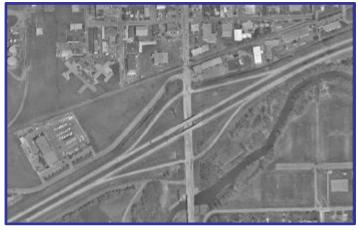
diamond interchange. The advantages of a single point interchange are the elimination of a traffic signal on Minnesota Avenue and the capacity to accommodate heavier traffic volumes. The adjacent full movement accent points located to the north and south of the interchange also impact the traffic operations along Minnesota Avenue.
