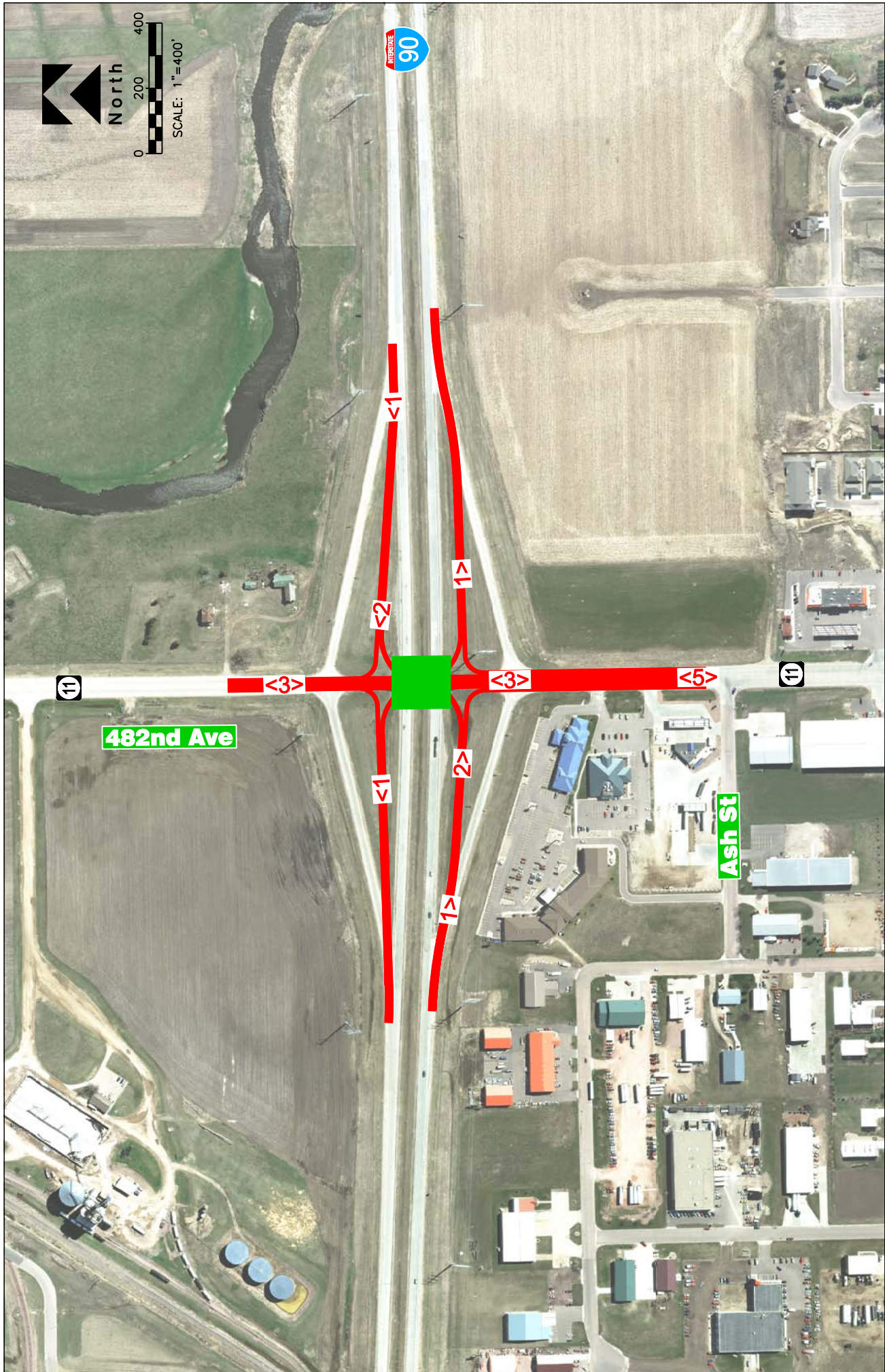
Figure 2 I-90 Exit 406 - Brandon/Corson Single Point Urban Interchange
