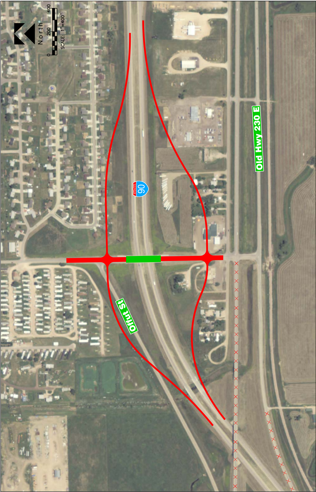
Figure 1 I-90 Exit 63 - Box Elder/Ellsworth AFB Diamond Interchange
