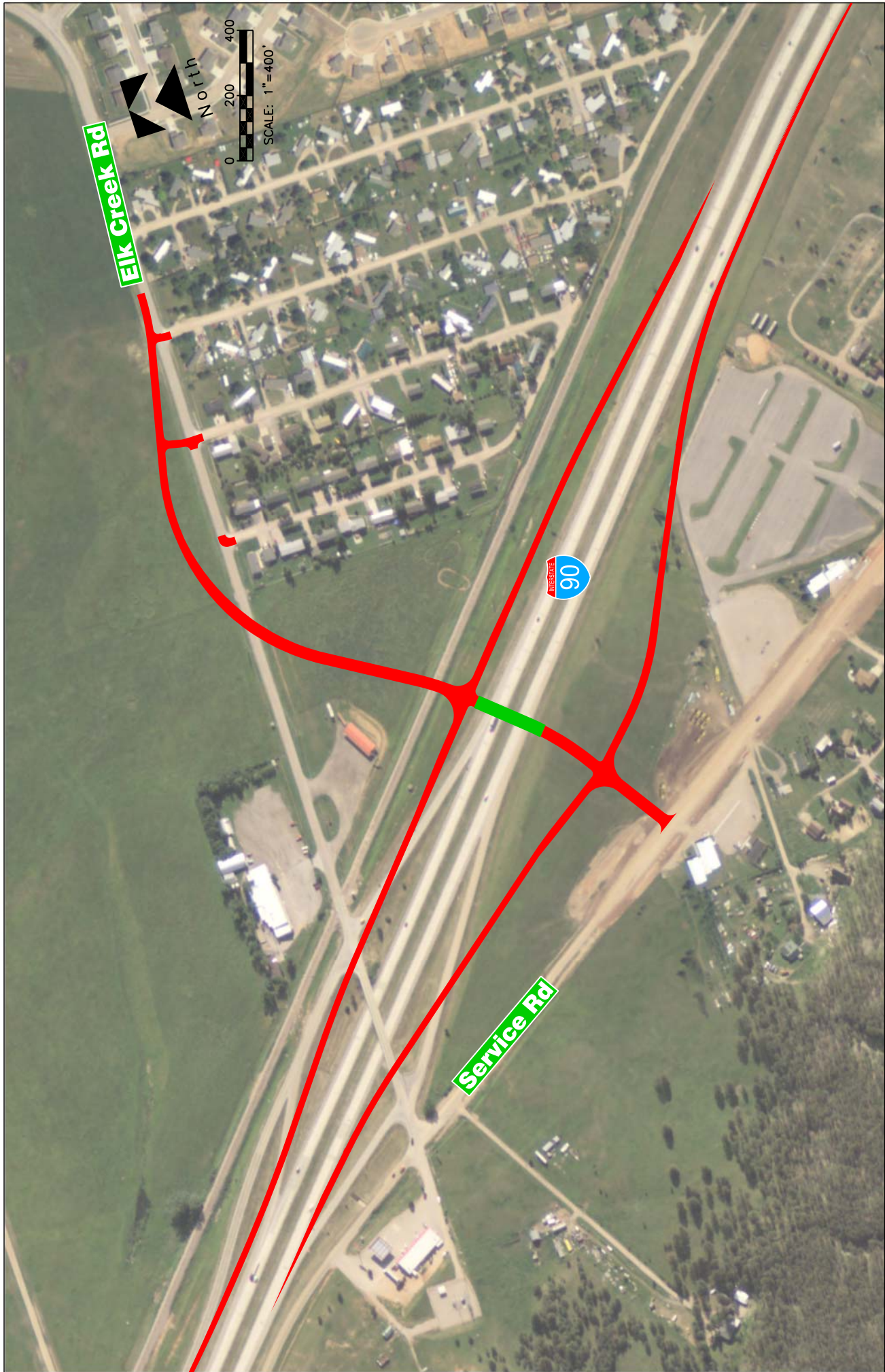
Figure 1 I-90 Exit 46 - Elk Creek Road, Piedmont Relocated Diamond Interchange
