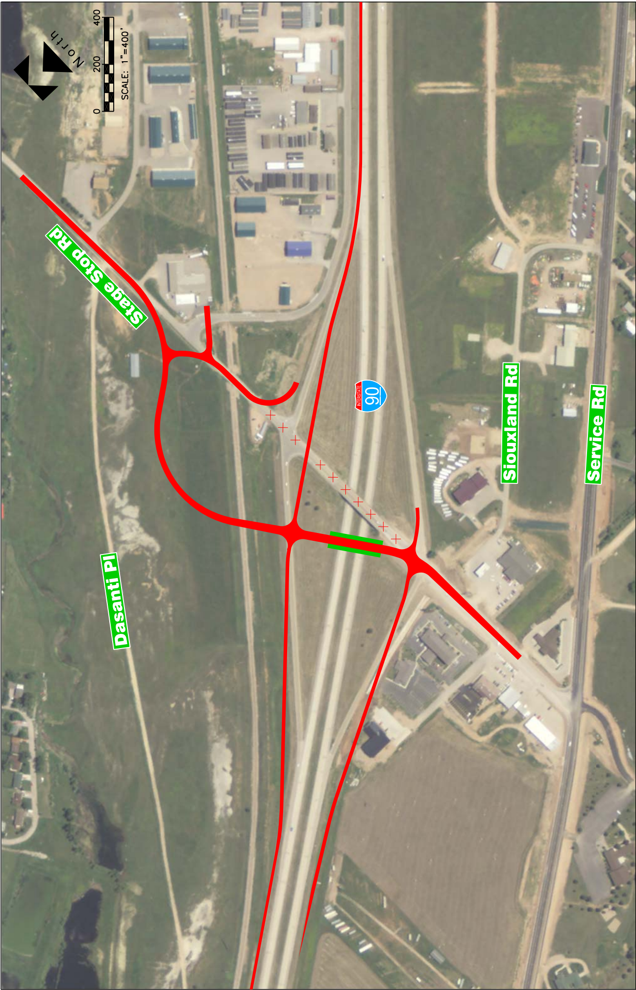
Figure 1 I-90 Exit 48 - Stage Stop Road, Piedmont Relocated Diamond Interchange
