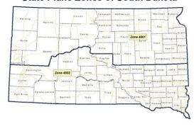
The State Plane Coordinate System (SPCS), is only used in the United States and is a plane coordinate system (north-south and east-west lines are perpendicular) in which each state has between one to six zones (South Dakota has two). This coordinate system's high level of accuracy is achieved using relatively small zones.
