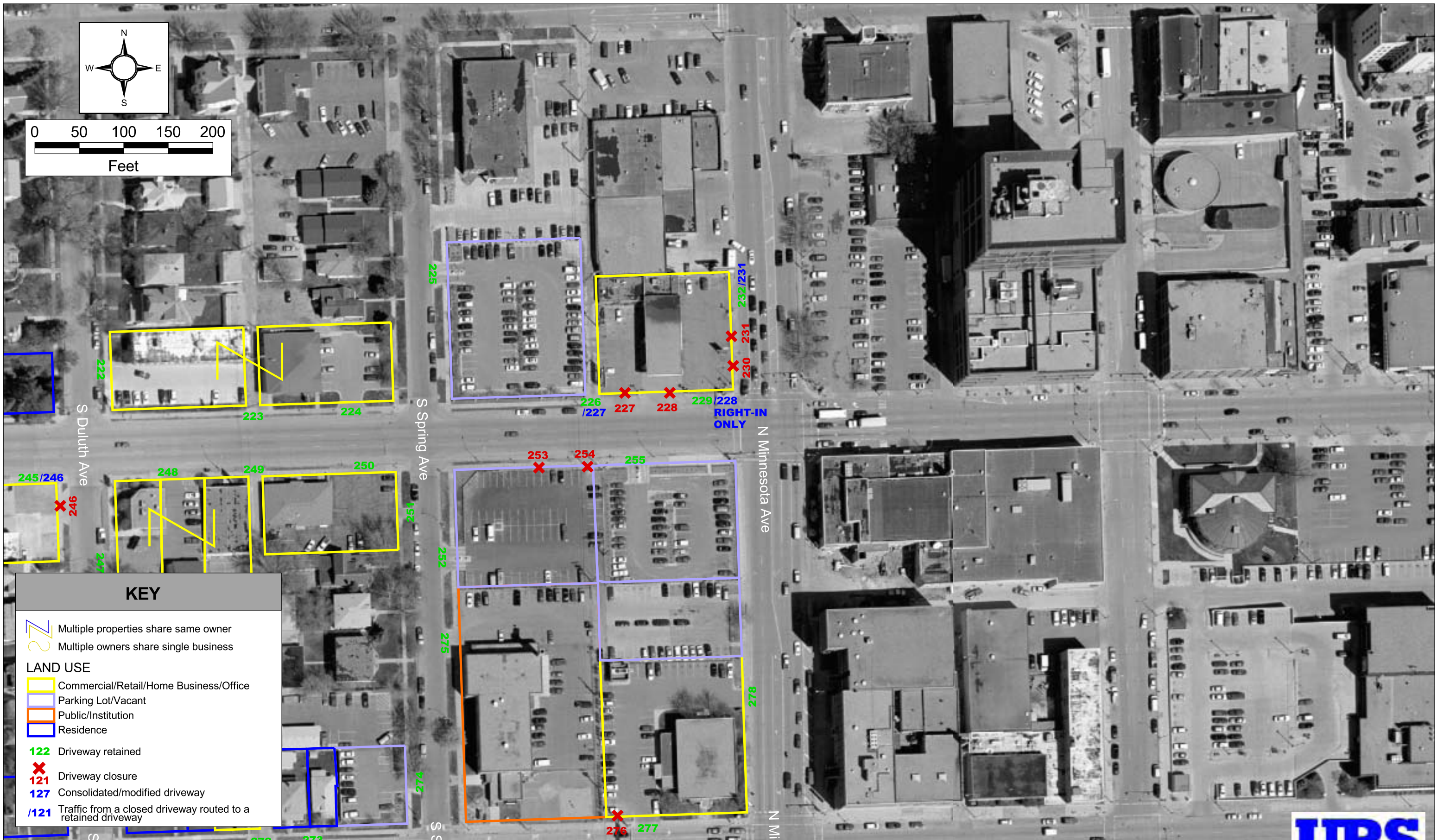
Figure 6-15 Initial Access Management Plan 10th Street: Spring Avenue to Minnesota Avenue
