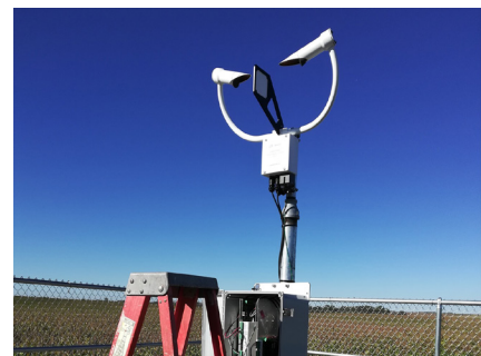
AWOS-III weather observing system.
