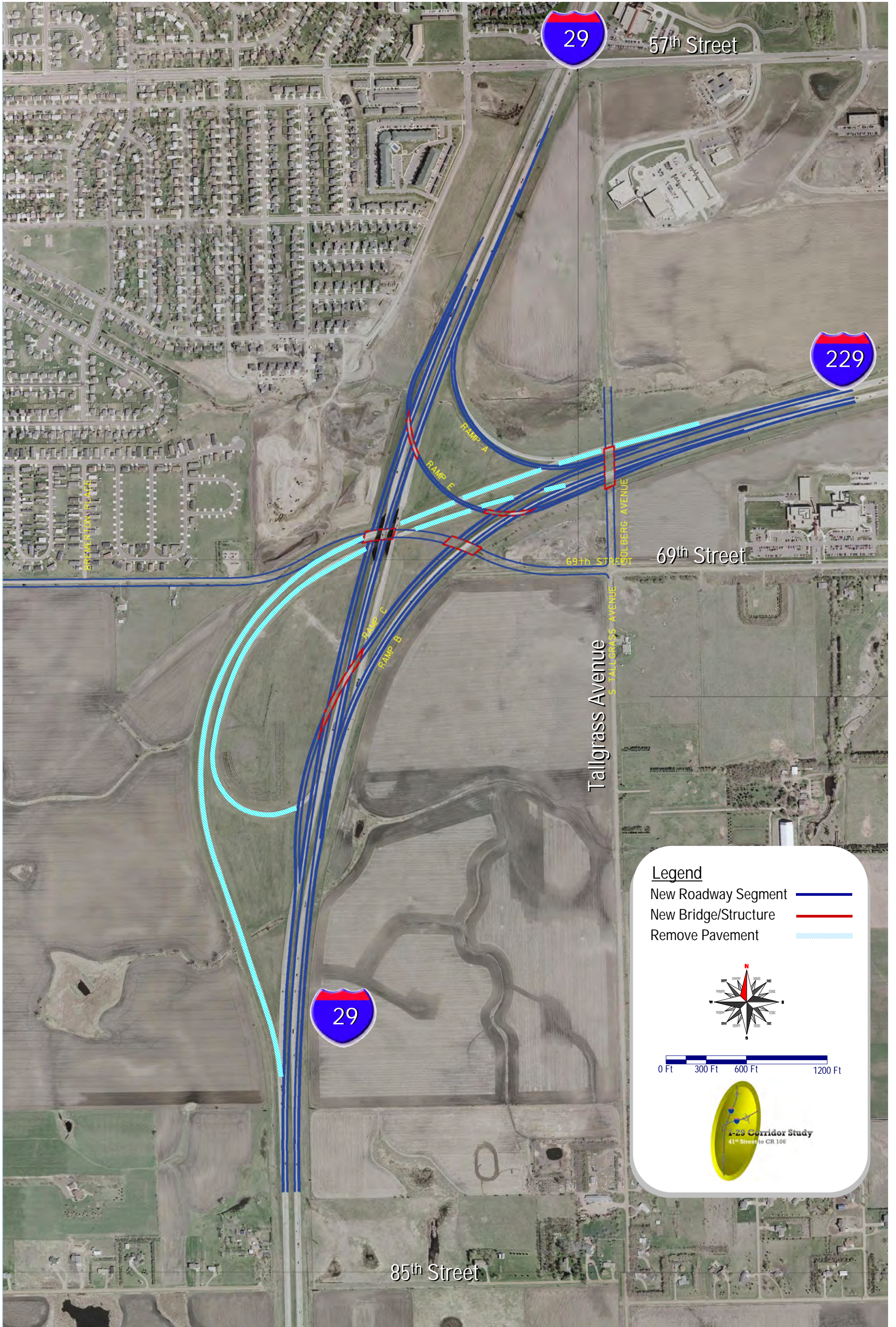
Figure Preliminary Interchange Concept – I-29/I-229 Completely Rebuild Directional Interchange – North 69 th Street Alignment (Overpass)
