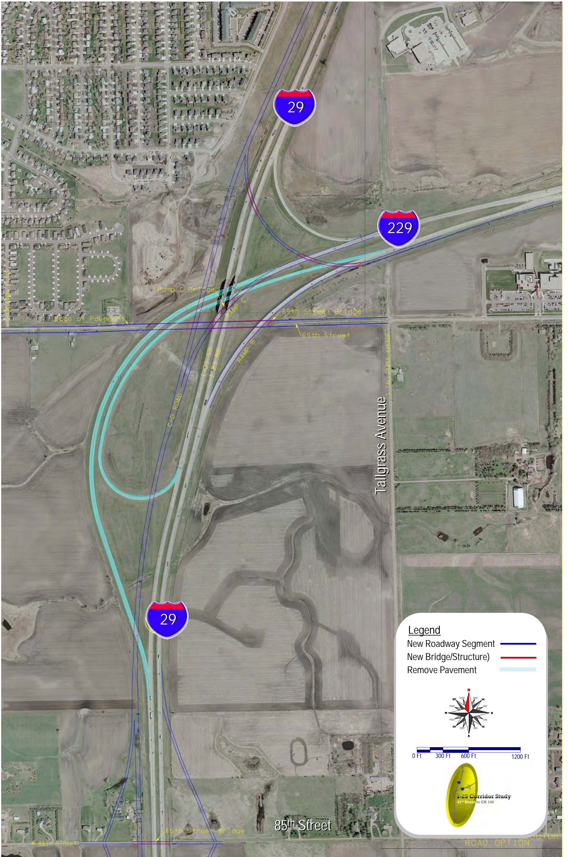
Figure Preliminary Interchange Concept – I-29/85th Street Diamond Integrated with Re-aligned Southbound I-29
