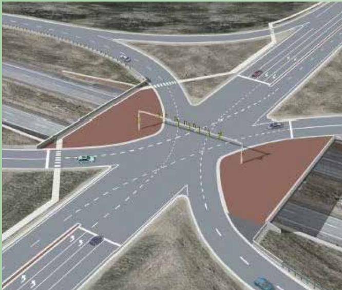
An illustration of how traffic flows over the new Interstate Highway 90 Exit 14 interchange at Spearfish
