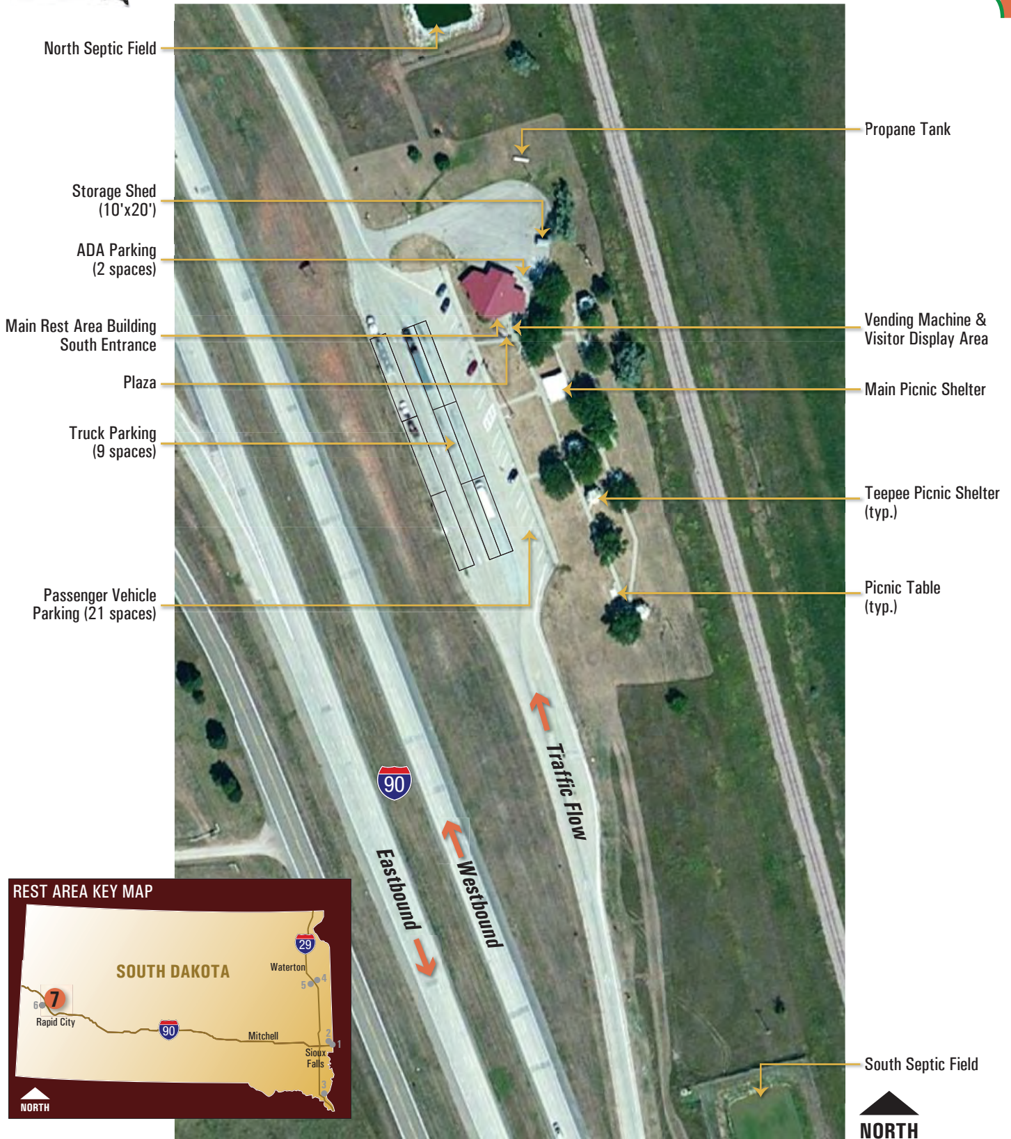
Figure 1. Tilford Westbound Rest Area Site Layout
