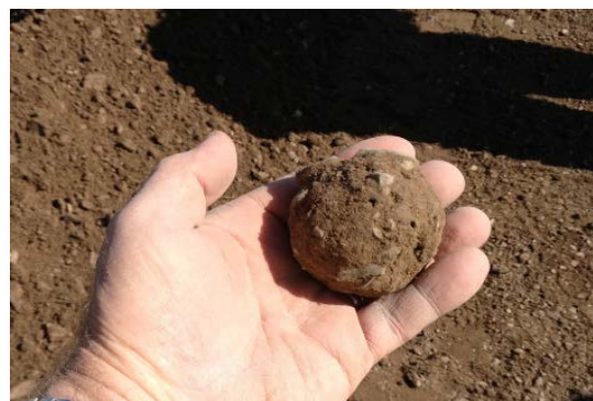
Field demonstration of surface gravel with an outstanding binding characteristic.
